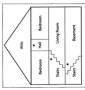
Install a smoke alarm and a carbon monoxide alarm (or combination alarms) in the basement and on each floor except the attic or a storage area.
